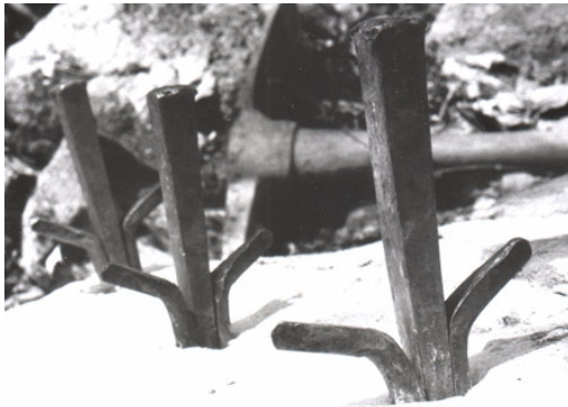
Wedges and shims in place
